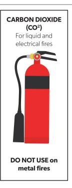
The contents of an extinguisher is indicated by a zone of colour on the red body. Halon extinguishers are not shown since no new Halon production is permitted in the UK.
