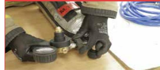
Pick up part 2 and screw part 2 into the threaded valve of part 1. The connection should be hand tight only.
