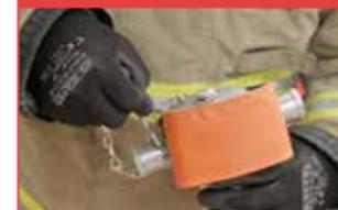
Place the split pin through the coupling lug by lining up the hole.
